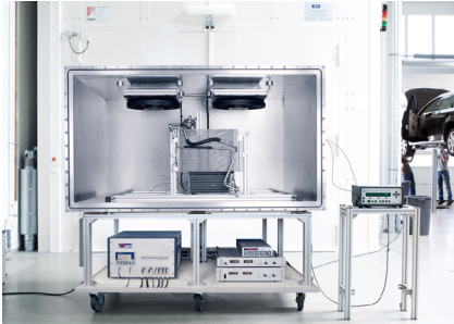
Figure 1: Test setup at IPETRONIK, Germany, with an evaporator air module. The Photoacoustic Gas Monitor INNOVA 1512 is mounted close to the MAC test bench.
