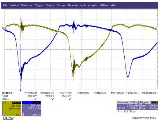
Figure 4. Crystal output magnetron to ground. Ch. 1: Magnetron A; Ch. 2: Magnetron B.
