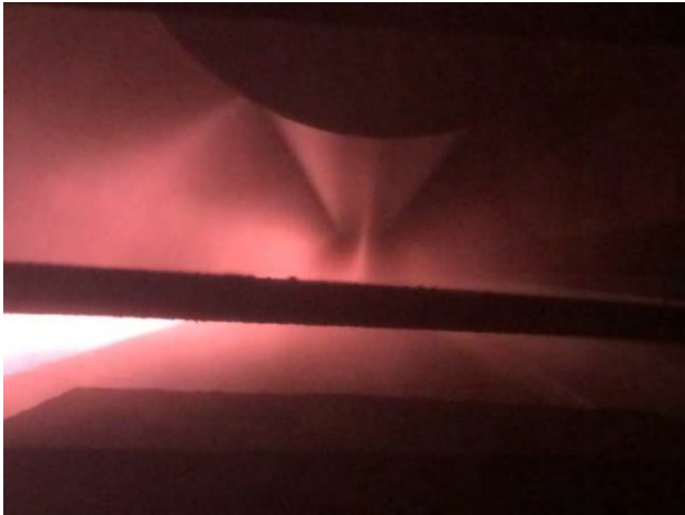
Figure 3. Unpowered magnetron affecting current flow.
